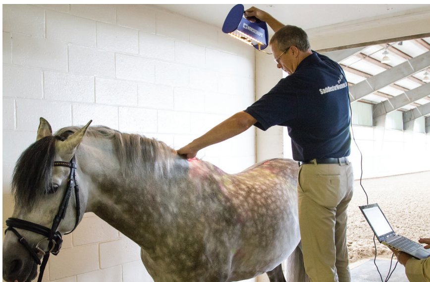
The HorseShape® laser captures the 3-Dimensional back shape with a computer printout that can be compared over time as the horse changes – photo used with permission.
