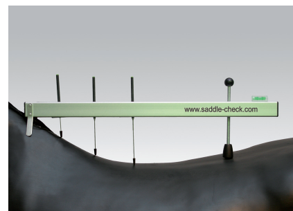
The BVFR uses this standardized but also somewhat unwieldy device to measure the horse's topline.
