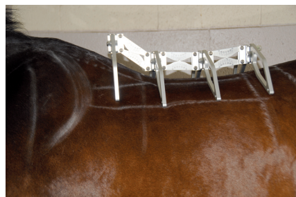
The Art Device (or "lobster claw") also measures the angulation all along the back.
