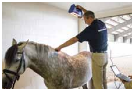
The HorseShape scanner replicates the exact shape of the horse's back and is used here to take just some of the many preliminary measurements necessary to build a saddle customized for any horse's unique requirements. Building a great saddle starts from the ground up or in our trade 'the tree up'.
