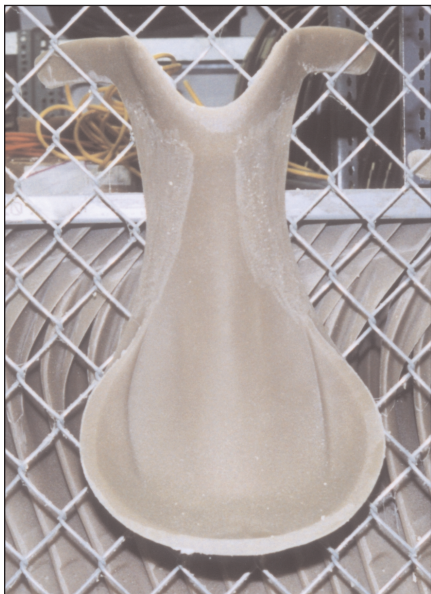
This tree is made from a lightweight material specially developed for Schleese Saddlery. A single tree weighs 2.75 lbs. Traditional ones are made from laminated beechwood and weigh 4 lbs.
