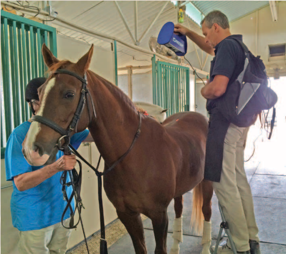
Jochen Schleeese uses HorseShape laser to determine horse's 3D back shape. Photo courtesy Schleeese
